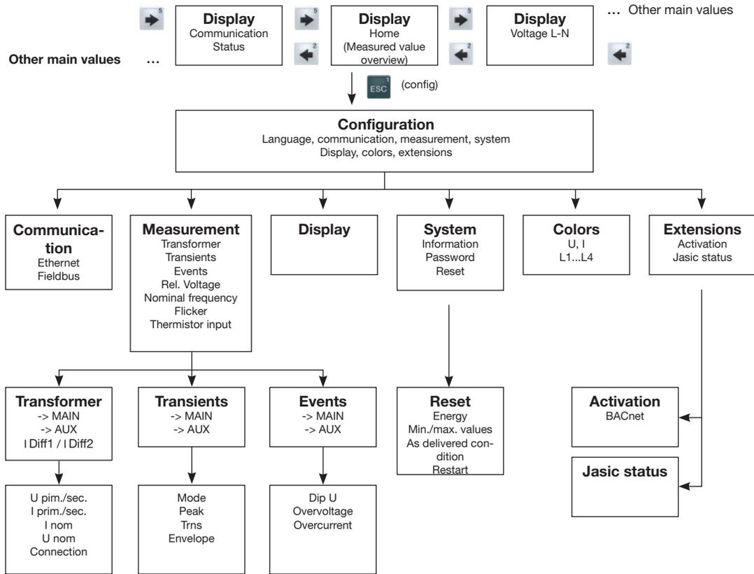
Fig. Schematic representation of the menu navigation for the configuration menu
