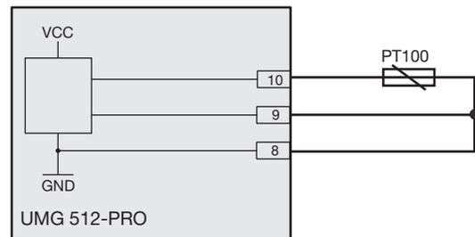
Fig. Schematic representation of the connection example
