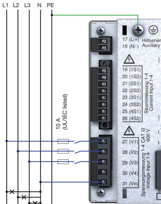
Fig. Connection example for voltage measurement.
