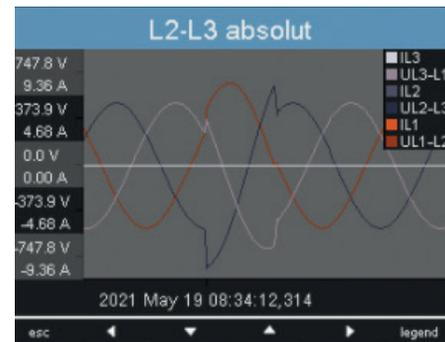
Fig. Display of a transient (VLL reference)
