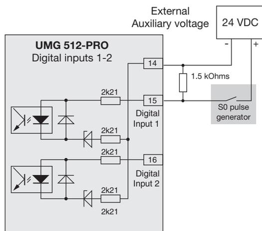
Fig. Example for the connection of an S0 pulse generator to digital input 1
