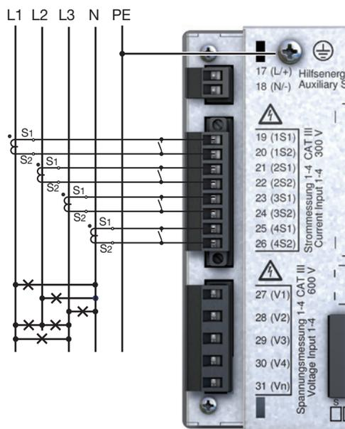
Fig. Connection example, "Current measurement via current transformer".
