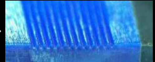
Glass deposition on V-groove
