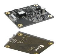
TRAX2 is the only orientation module that provides two different modes: AHRS or digital compass. TRAX2's dual-mode capability supports a wide range of applications including drones, robotics, ocean buoys, manned and unmanned vehicles, among others.
