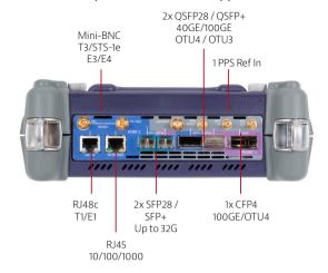
2x SFP+/SFP28 1-10-25G Ethernet LAN/WAN OTN 1-1e/2/2e STM-1-64 & OC3-192 Fibre Channel: 1,2,4,8,10,16G, 32G FC CPRI 614M — 10.1, 24.3G
