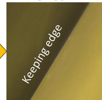
**Blade edge after cleaving 250um fiber 10000 times**
