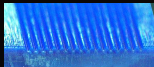
Glass deposition on V-groove
