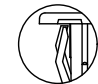
DETAIL VIEW VHP CONTURA VII, VIII & IX HOLE PLUGS (No wing serrations for ease of removal)
